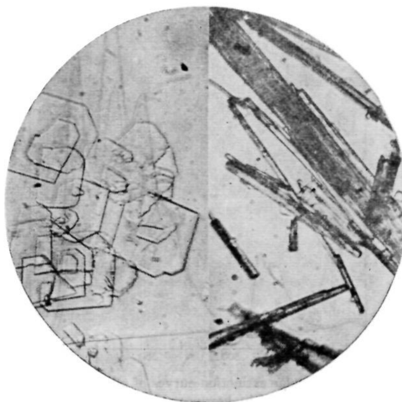
Fig. 7.—Crystals of all-trans -diphenyloctatetraene (plates), and of the cis -I form (prisms). From chloroform-methanol; 430 X.
